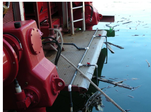
Nitrogen is applied from the tanker truck via pipes off the back of the barge and mixed into the water column by the prop wash.
