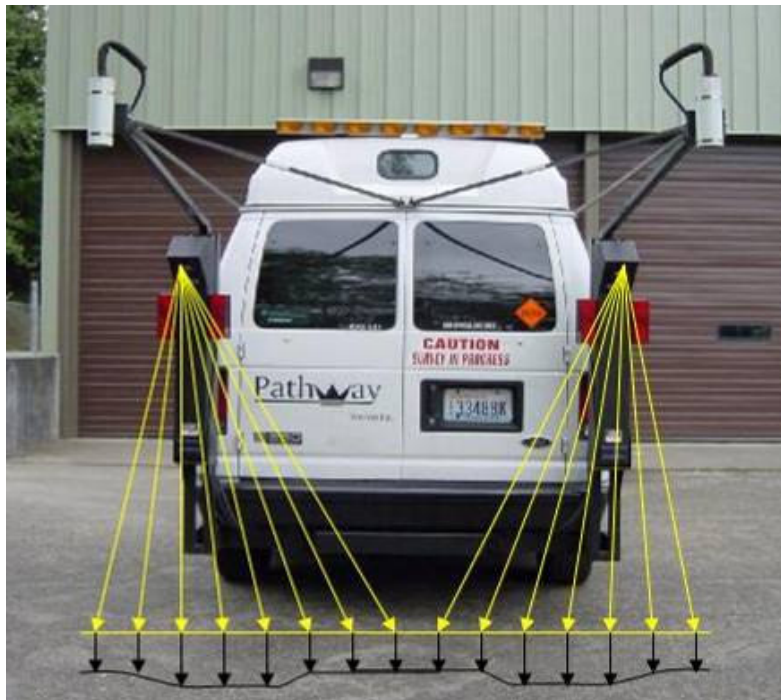
Photo 16. High speed WSPMS van and schematic of rut/wear depth determination.
