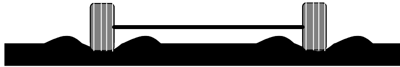
a. HMA shoving due to trucks
